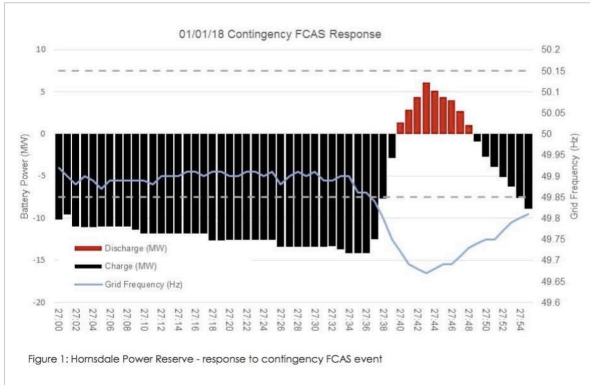
A 100 MW battery that is charging can deliver a 200 MW change in the balance between demand and supply, almost instantaneously.
